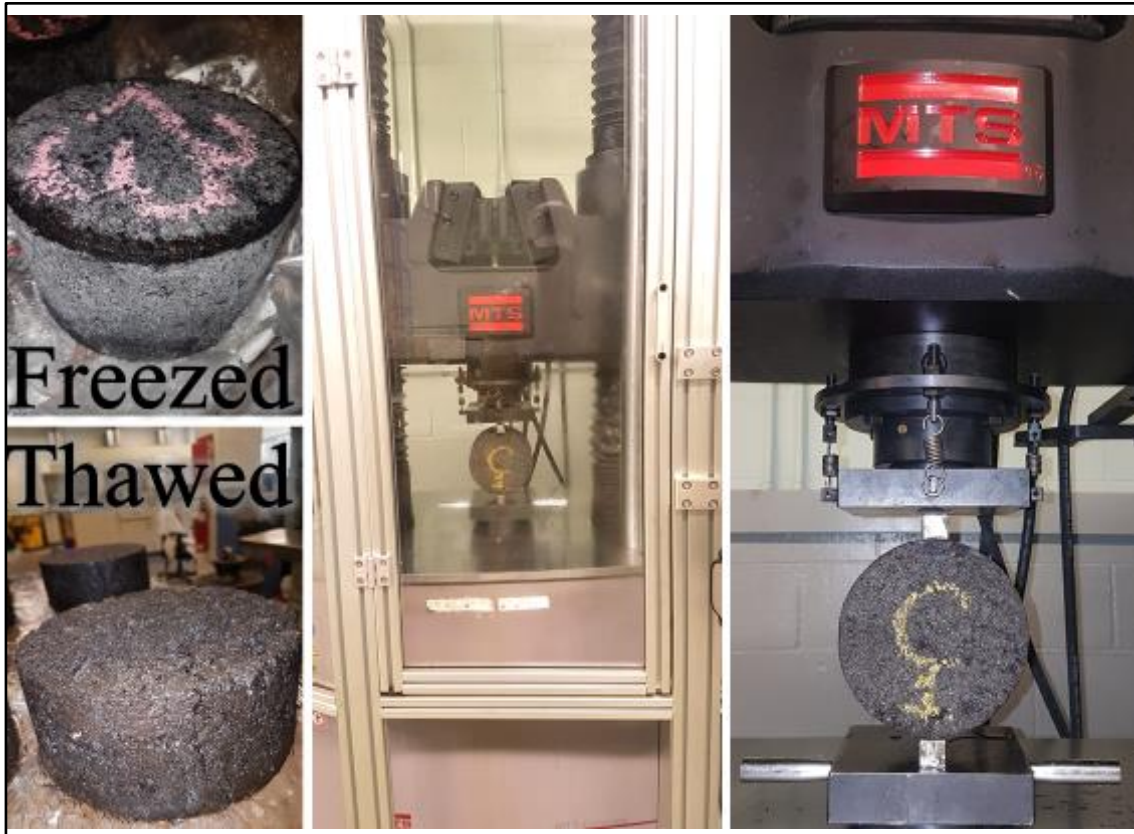
Figure 2.13 Tensile Strength Ratio Conditioned Samples and Compaction Equipment
